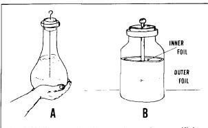
fig. 1. (A) An example of a capacitor such as von Kleist discovered; (B) A Leyden jar (occasionally called a "Kleistian jar). and studying electricity. In doing so, he unwittingly discovered the world's first electrical "condenser" or capacitor. And believe it or not, this discovery led to antennas as we know them today.
